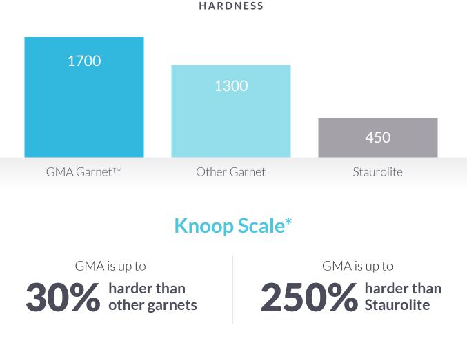
\*The Knoop scale is a measure of the hardness of a material.
