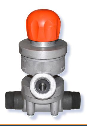
The original Thompson Valve is a normally closed, self sealing, abrasive metering valve known for its instant, smooth response to either pneumatic or electric deadman controls. This fail-safe valve shuts off abrasive flow to the nozzle and seals the tank at the same instant. A remote abrasive cutoff is available, allowing the operator to stop the flow of media while continuing a constant flow of air. This provides a quick and easy way to clear the blast hose and blasting area of abrasive.
